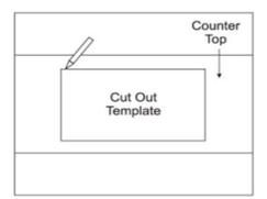
Move out the template and cut along the countertop based on the made line using appropriate cutting tool.
