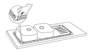
Move the sink out of the countertop and draw another line with inner spacing 10 mm (1 cm) from the first line. Drill all four corners with a hole and cut along the countertop following the second line. (Another option is to use the "cut-out" dimension that provided through the label attached on the product).
