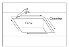
8. Tighten the screws carefully and remove the leftover sealant around the sink.
