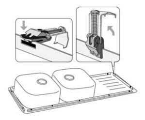
5. These anchor brackets are designed to be used with 30 - 40 mm thick countertop (1). If the countertop is thinner, insert the wooden wedges between the countertop and the brackets to secure them (2). After installing two brackets at each corner, install the rest evenly spaced around the perimeter of the sink.
