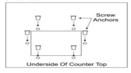
Place the fixing brackets over the screw anchors. Insert the provided screw, but do not fully tighten it.
