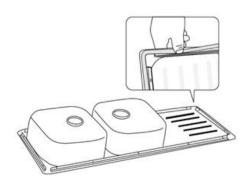
4. Install the anchor bracket vertically underside the sink and pull the up to lock into their horizontal position.
