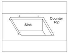
Apply sealant to the suitable wet area that recommended for stainless steel sink and countertop material.
