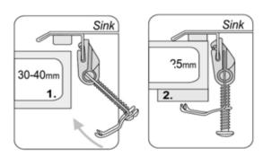
6. Tighten the screws of the anchor brackets to secure the sink in its place.
