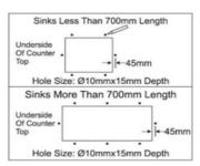
4. Insert screw anchors into the drilled holes.
