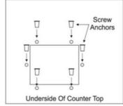
5. Place fixing brackets over the screw anchors. Insert the screw provided, but don't fully tighten.
