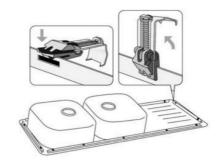
5. These anchor braces are designed for use with countertop 30 - 40 mm thick (1). If the countertop is thinner, insert wooden wedges between the countertop and the braces to secure them (2). After placing two at each corner, place the rest evenly spaced around the perimeter of the sink.
