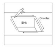
8. Tighten the screws carefully and remove the excessive sealant.
