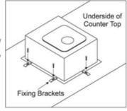
6. Check alignment between the bowl and the cut out hole.
