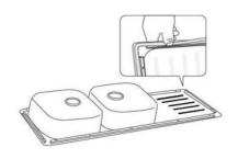
4. Place the anchor braces vertically and pull the up to lock into their horizontal position.
