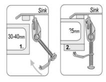
6. Tighten the screws of the anchor braces to secure the sink in place.
