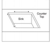
7. Apply suitable wet area sealant recommended for stainless steel sink and countertop material.
