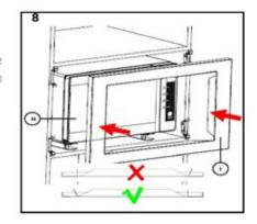
9. Ensure the frame microwave installed correctly and neatly.
