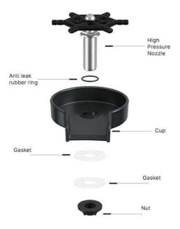
1. Assembly the high pressure nozzle to the cup:
