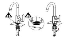
3. Connect the hot water and cold water hoses, and then tighten them with a wrench.
